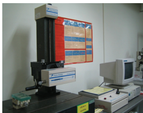
Figure 2 The machine for surface measurement (Form Talysurf series 2®, Rank Talor Hobson Leicester, England)
