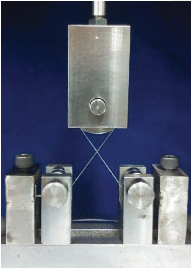
Figure 1 Forming general purpose stainless steel wire to archwires.
