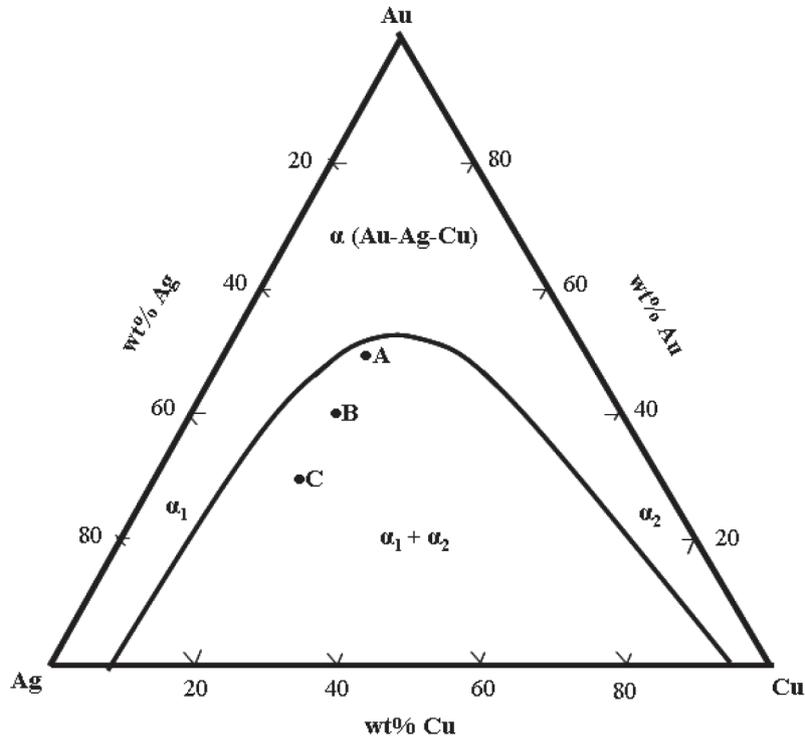
**Figure 1** Au-Ag-Cu isothermal section at 700°C (A: 50Au-30Ag-20Cu alloy, B: 40Au-40Ag-20Cu alloy, and C: 30Au-50Ag-20Cu alloy)<sup>6</sup>
