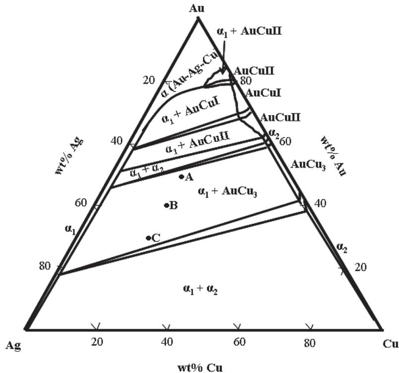
**Figure 2** Au-Ag-Cu isothermal section at 300°C (A: 50Au-30Ag-20Cu alloy, B: 40Au-40Ag-20Cu alloy, and C: 30Au-50Ag-20Cu alloy)<sup>7</sup>
