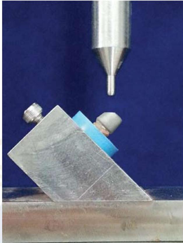
**Figure 3** Mounted specimen with the custom-made jig assembled to the universal testing machine
