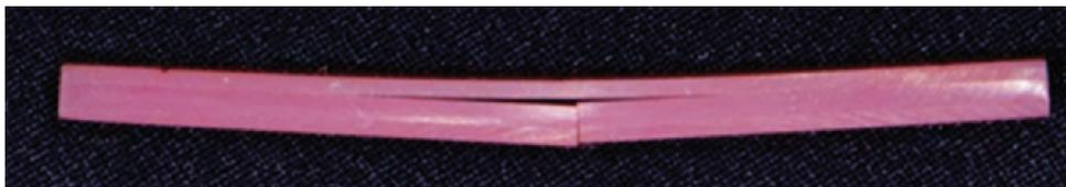
Figure 3. De-bonding of Kooliner from ProBase Hot after flexural strength test
