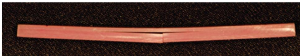
Figure 4. De-bonding of Tokuyama Rebasell from ProBase Hot after flexural strength test
