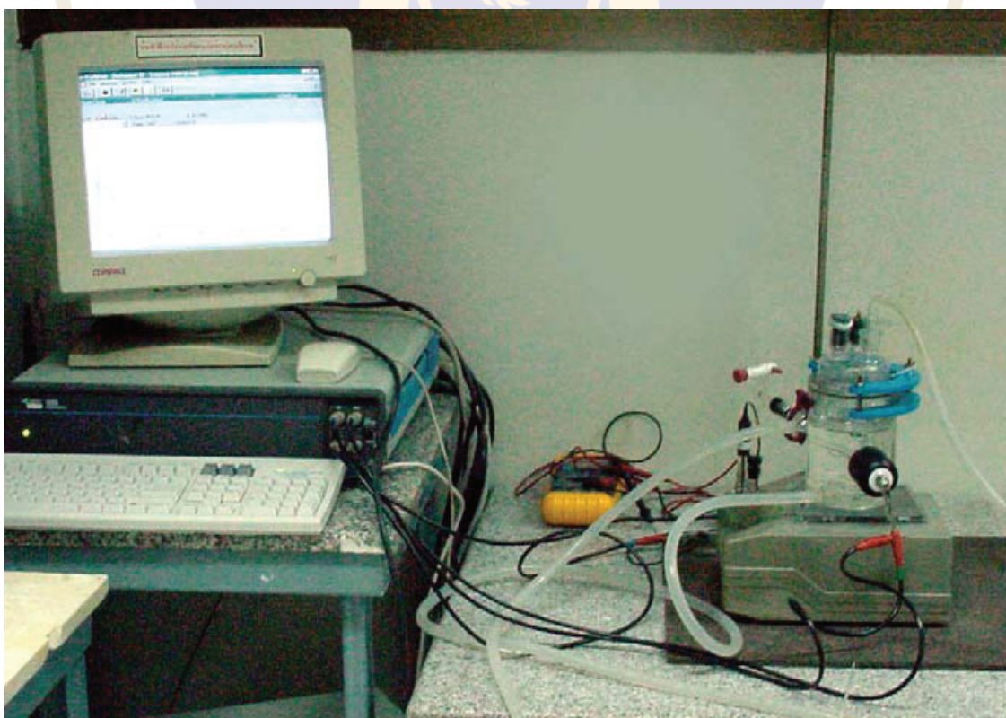
Figure 2 Electrochemical cell and polarization system
