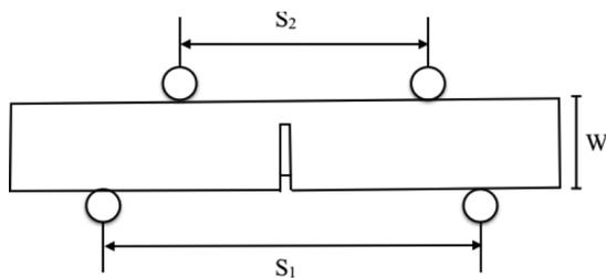
**Figure 3** Test specimen for fracture toughness with Chevron Notch
