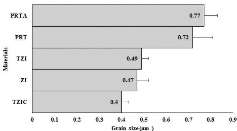
**Figure 4** The grain size ( $\mu\text{m}$ ) of five zirconia groups.
