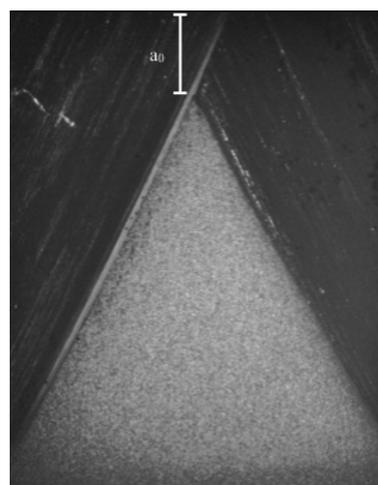
**Figure 2** SEM micrographs showing the fracture surface of zirconia specimen with chevron notch after testing.
