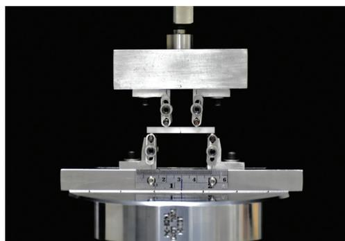
**Figure 1** Load configuration under four-point bending test.
