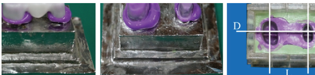
Figure 2. Silicone replica technique : Low-viscosity silicone is loaded at the fitting
