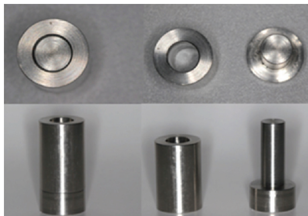
Figure 1 Split circular shaped stainless steel mold.
